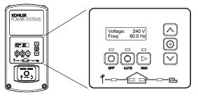
The RDC2 controller provides integrated control for the generator set, Kohler<sup>®</sup> Model RXT transfer switch, programmable interface module (PIM), and load control module (LCM).
